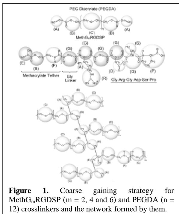
together and represented by a super bead with the mapping point being taken as the center of mass of each group of atoms. Fig. 1 illustrates the strategy used to coarse grain the two types of crosslinkers (PEGDA and MethG<sub>m</sub>RGDSP) and the copolymer network formed by them. The water molecules were also represented by a CG scheme, in which four water molecules represented by
