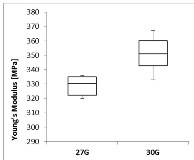
Figure 1. Young's modulus of PCL fibers 3D printed with two different needle gauges, 27G and 30G.
