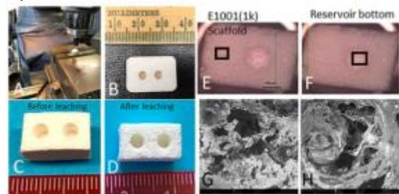
Figure 2. Scale up of porous scaffolds with machined reservoirs. SEM imaging of the bottom of the reservoirs was performed and displayed minimal deformation of the pore structure.
